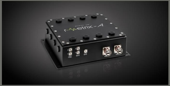
Solid State CPU with GPS, Wi-Fi, Ethernet, and Cellular
